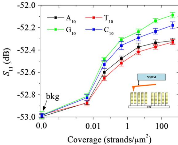
**Fig. 1.** The change in the microwave reflection coefficient,  $\Delta S_{11}$ , as a function of coverage of 10 mer A, G, T, and C probes. The inset shows the schematic picture of oligonucleotide probes and the NSMM tip.
