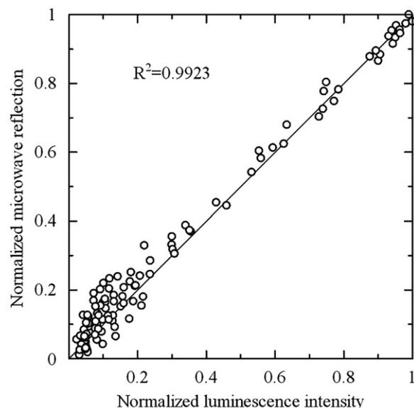
**Fig. 5.** Correlation of the normalized microwave reflection coefficient with fluorescence amplitude for spots in the hybridized Agilent 44k microarray.  $S_{11}$  was normalized to the slide substrate as background, while fluorescence intensity was normalized to the highest measured signal.
