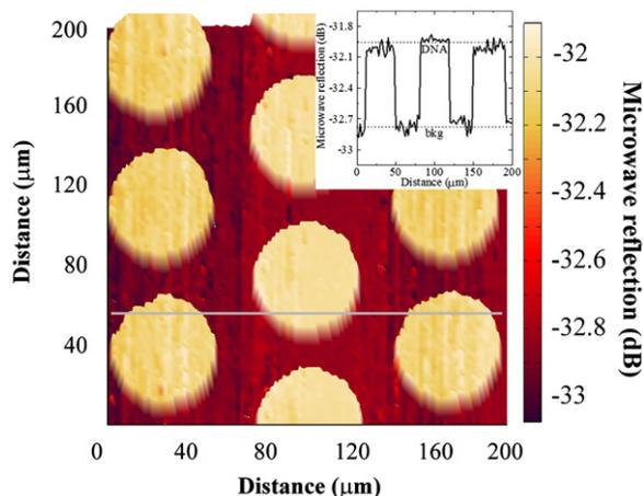
Fig. 3. 3D NSMM image of unhybridized 60-mer probe Agilent 44k DNA microarray. Image area was  $200 \times 200 \mu\text{m}^2$  and scanning resolution was  $2 \mu\text{m}$ . The inset shows the cross sectional profile indicated by the solid line in the 3D NSMM image.
