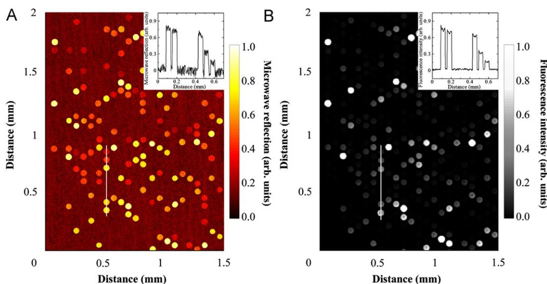
**Fig. 4.** (a) 2D NSMM map (with 2  $\mu\text{m}$  scanning resolution) and (b) fluorescence image (prepared by Agilent Technologies) of the hybridized 60-mer DNA microarray. The same position with 1.5  $\times$  2  $\text{mm}^2$  surface area of the microarray is shown in both images. The insets show the corresponding cross sectional profiles along the solid lines in each image.
